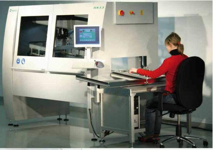
The soldering system is equipped with a multi-stage glass ceramic pre-heating system, specially developed for subassembly production.
